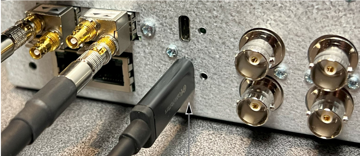
Thunderbolt 3 option module installed in MTRX II, Thunderbolt 3 cable connected
