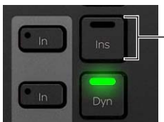
Inserts switch on Process Module
