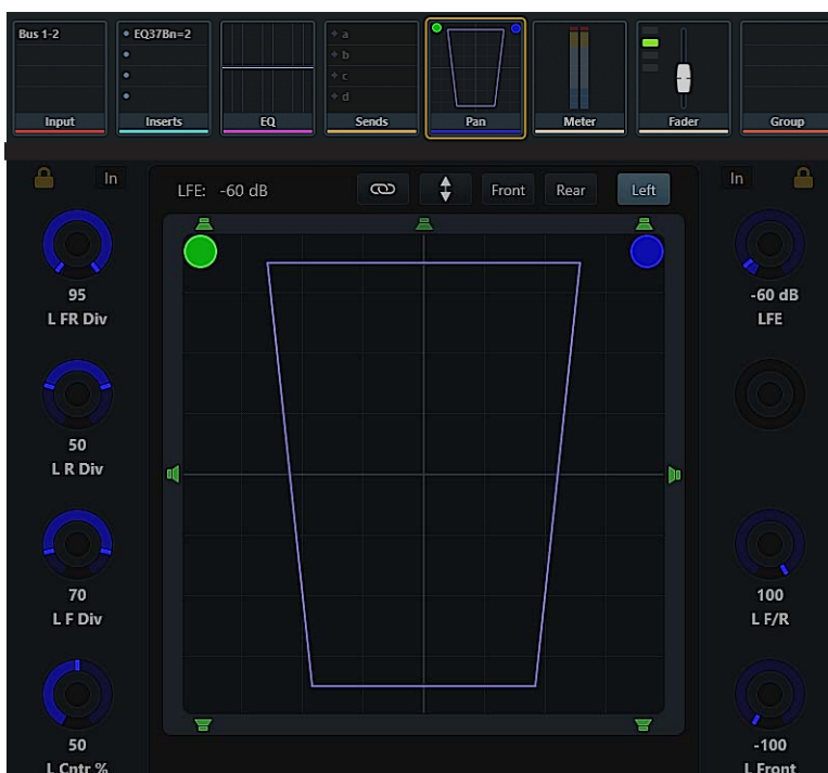
Figure 82. Surround panner on the touchscreen when a stereo track is assigned to a multichannel output path.
