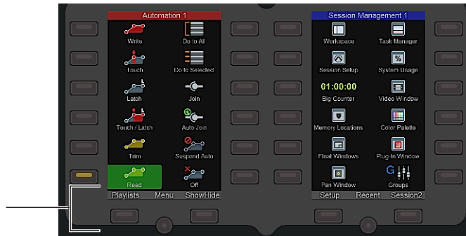
Navigation switches along the bottom of the left Soft Key bank on the Master Module (default Pro Tools appset)
