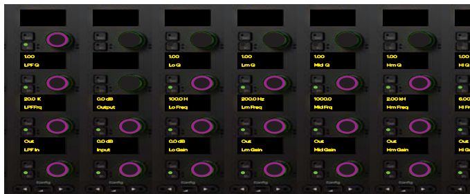
Figure 108. Attention Expand Knob Zone with expanded EQ3 7-band (plug-in bypass via column 8 Back switch)
