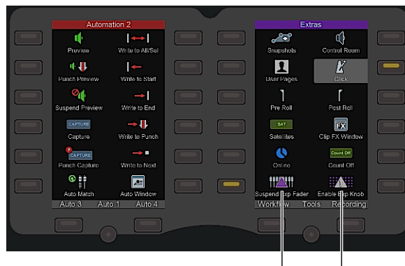
Figure 110. Automation Module Soft Keys showing Attention Expand Faders enabled and Attention Expand Knobs disabled
