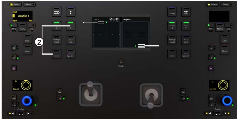
MJM panner grid in Height Adjust mode; a mono track at front/center, Height at minimum (0) / joystick 2 all the way down
