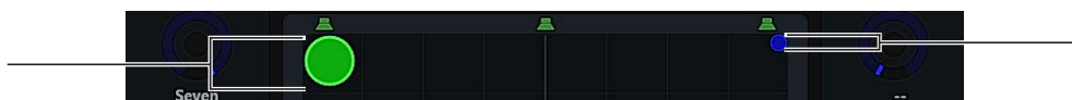
A signal at maximum Height (large green pan dot, Left) and minimum Height (small blue pan dot, Right) in standard 2D Pan view
