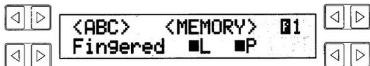
This display shows the current A.B.C. mode and Memory settings.
