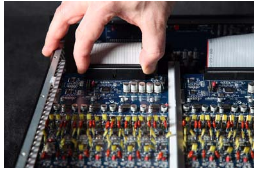
Removing the 50-pin cable connector from an I/O card
