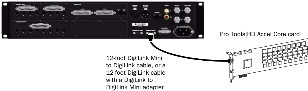
Figure 1. HD I/O connected to the DigiLink Port on a Pro Tools|HD Accel Core card (16-channel I/O system)
