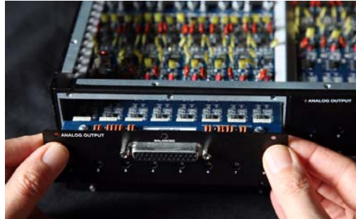
Removing an I/O card from the HD I/O chassis
