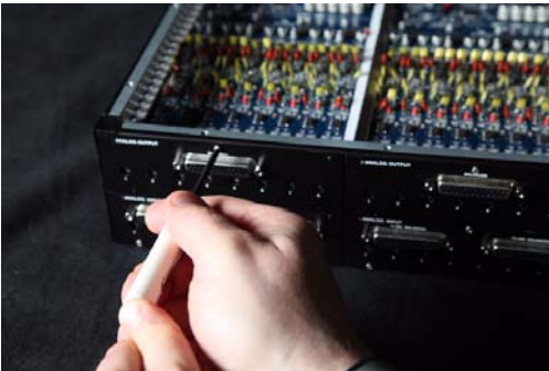
Removing the screws securing an I/O card
