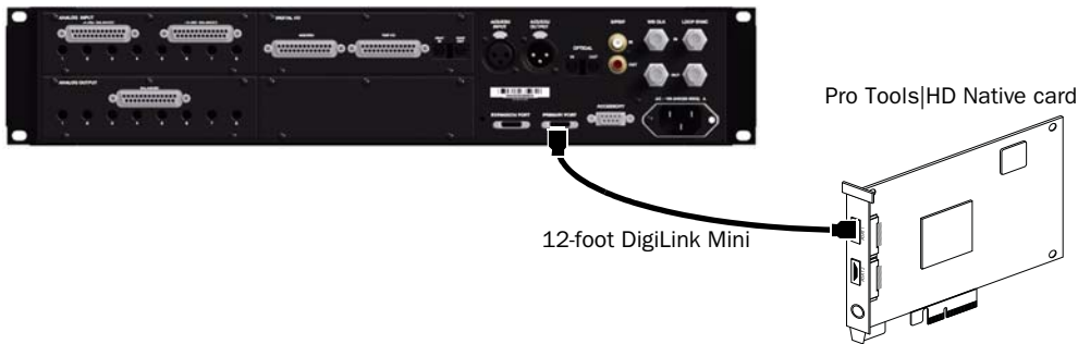
Figure 3. HD I/O connected to the DigiLink Mini Port 1 on a Pro Tools|HD Native card
