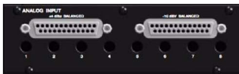
+4 dBu and -10 dBV DB-25 Analog Input ports
